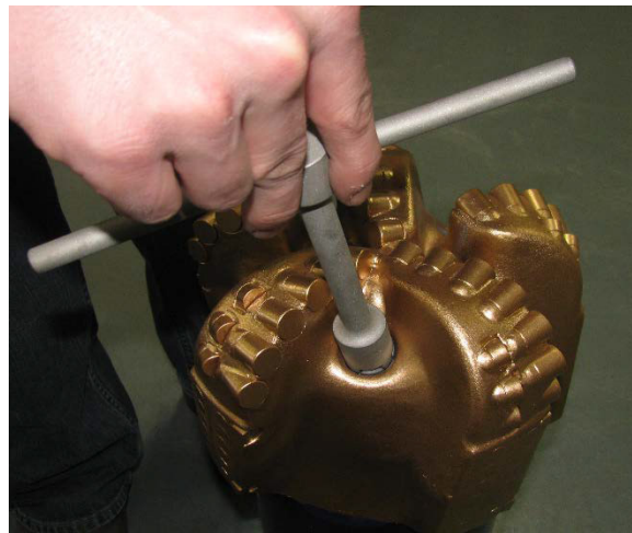
Figure 10. Use Wrench to Bottom Nozzle
