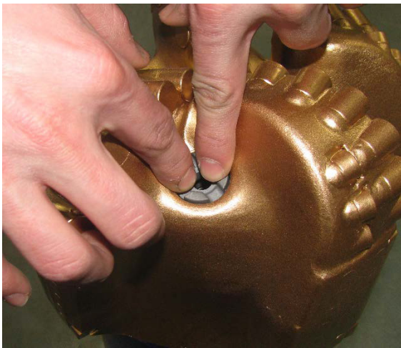
Figure 9. Hand Tighten Nozzle
