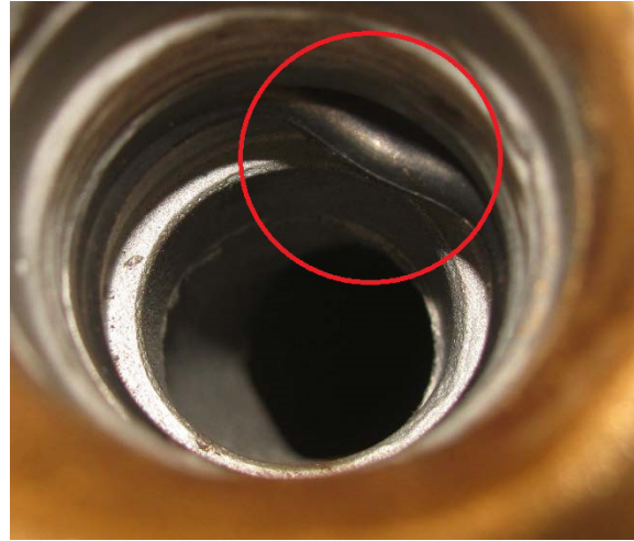
Figure 6. O-Ring Not Seated
