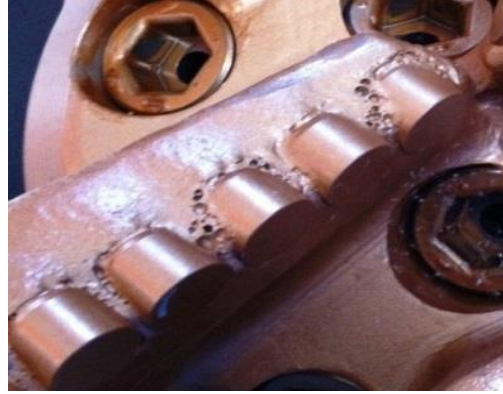
Excessive Braze Bubbling
